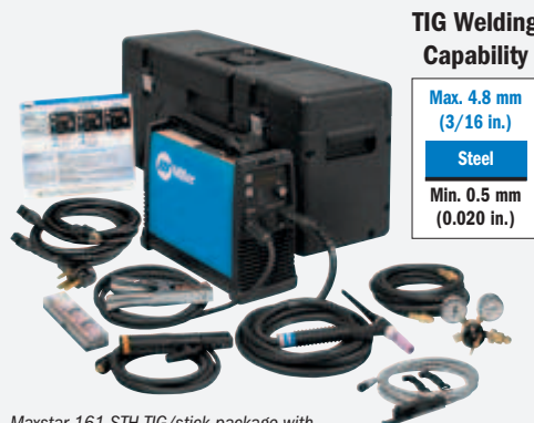
Maxstar 161 STH TIG/stick package with remote fingertip control (907711001) shown — includes X-CASE.
