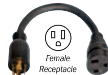
Twist Lock Adapter Cord 301489 For Fusion. L14-30R to NEMA 6-50R. Adapts engine drive 120/240-volt twist lock plug to common Milleromatic and Spectrum 240-volt plug.
