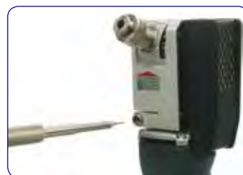
Precise adjustment of the stick-out
